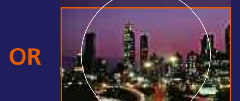
16:9 Centre Cutout Lossy. Uses just the central information for the 4:3 image. Important that original HD material is shot with this type of display in mind (Shoot to Protect)
